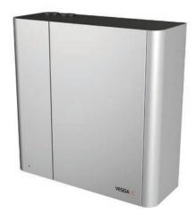
The VESDA-E VEA Local Relay StaX allows signaling of alarm location from the detector via relays and provides mounting of fire panel loop input modules inside the enclosure. It is directly powered and controlled from the detector. Depending on the configuration a VEA detector can power and control up to three (3) Relay StaX. Each Relay StaX provides 40 relay connections corresponding to 40 tubes on a VEA detector providing full addressability.
